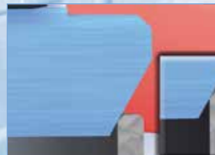
“Cut-off effect” – the conical shape of the marginal seat causes surface deposits to be removed during sealing
