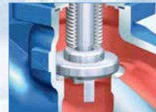
Additional stem guide via the V-port plug (permits higher differential pressures)
