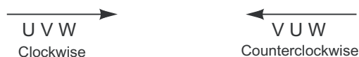
Figure 3-5 Direction of rotation of the motor when looking at the drive end
