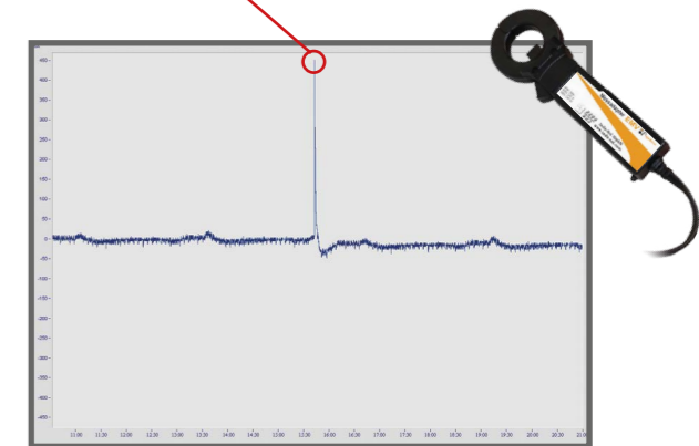
High-frequency glitch at the central supply 24 VDC
