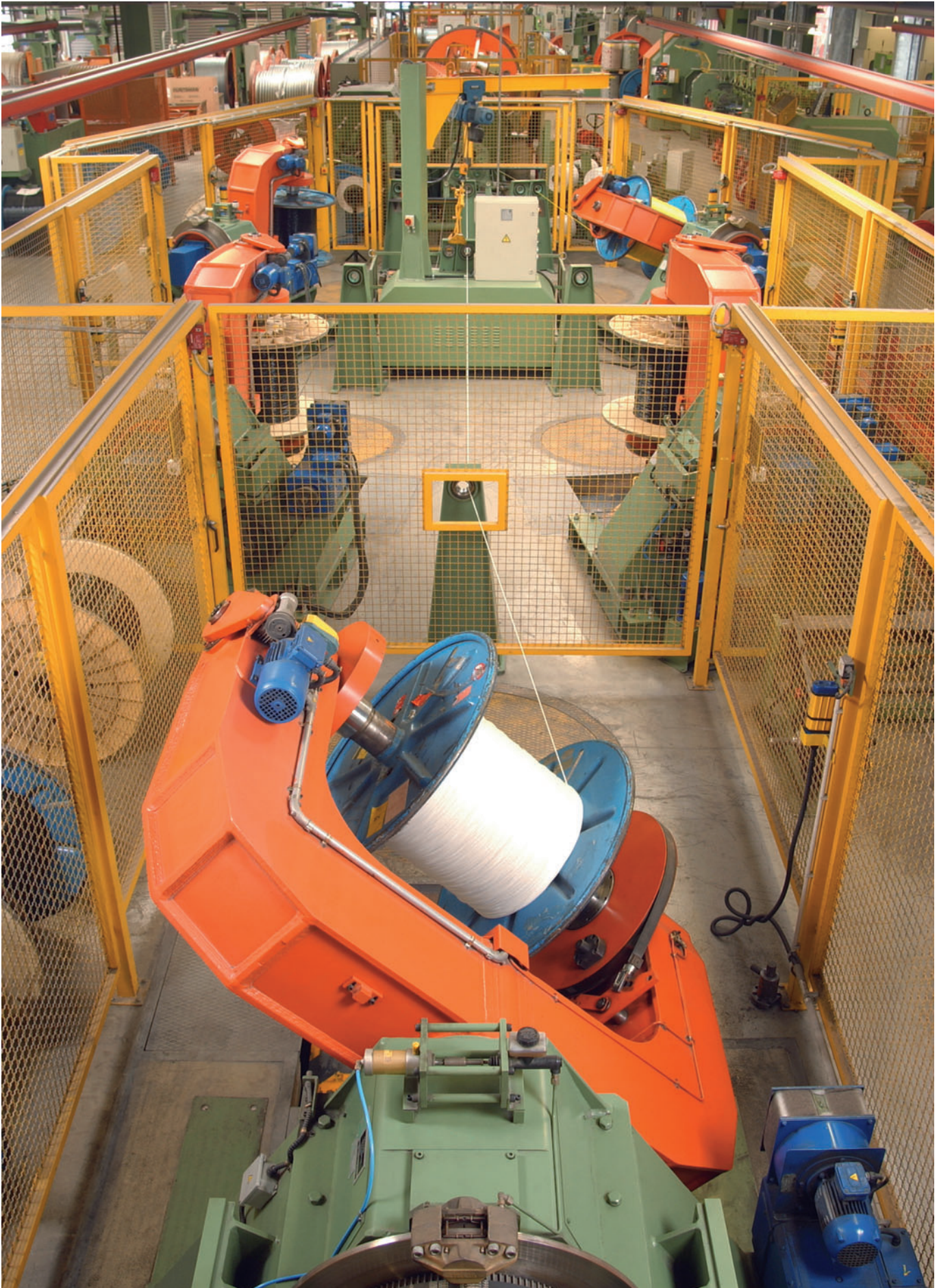
Large cabling machine with backtwist at our Windsbach factory
