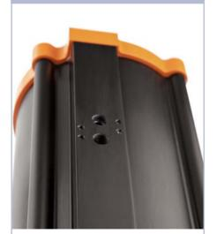
The NAMUR interface for direct mounting of control valves and the air ducts integrated into the housing reduce the mounting and tubing required to a minimum.
