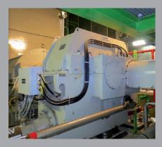
Each product is tested individually on one of our state of the art test bench at full speed condition, partial load test or even back to back locked torque test.
