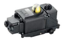
AMTRONIC is an open/close control unit suitable for mounting to ACTAIR/DYNACTAIR actuators from KSB with direct compressed air supply. It can be mounted either to quarter-turn actuators with VDI/VDE 3845 interface or linear actuators with NAMUR interface.
